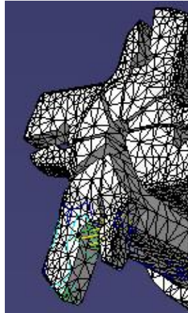
Figure 7. Clamping system with top clamp realized by two crossed spits in the tool body and a screw
