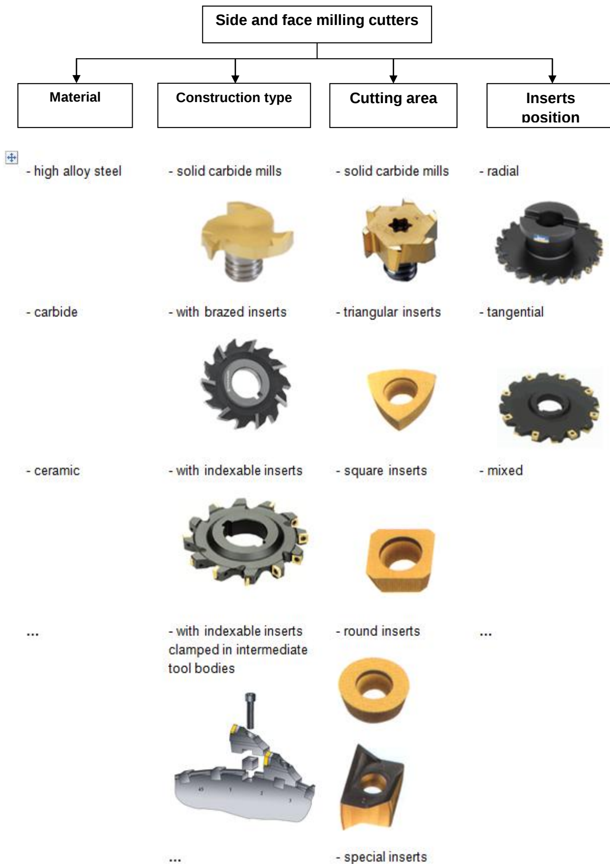
Figure 1.a Tree structure of the side and face milling cutters [4,5]
